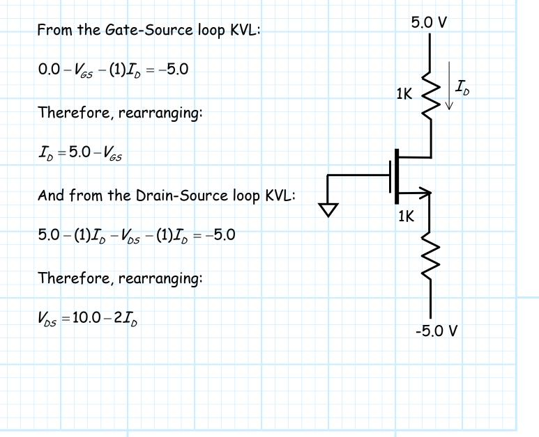
Look! We can equate the NMOS device equation and G-S equation to find  $V_{GS}$ .
