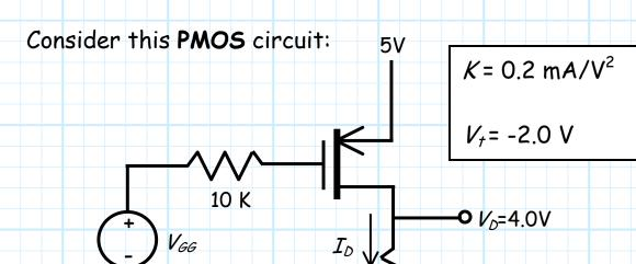
For this problem, we know that the **drain voltage**  $V_D$  = 4.0 V (with respect to ground), but we do **not** know the value of the voltage source  $V_{GG}$ .
